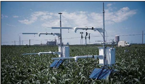
*Bowen Ratio Systems calculate evapotranspiration and CO<sub>2</sub> fluxes over a sorghum field near Lincoln, Nebraska.*
